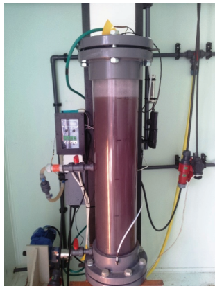
Fig. 3. Nutrient recovery and tests with pharmaceutical micro-pollutants to investigate contamination of the produced struvite fertilizers
